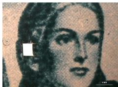
An analysis of a stamp by XRF was done by John Dale of Intertek MSG. This involves excising a sample from the specimen, bombarding it with X-rays in a vacuum (and in a very expensive box!) and measuring the emitted radiation. The ear was chosen since it has the densest colour.
